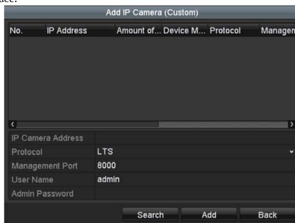
Figure 2. 14 Custom Adding IP Camera Interface
