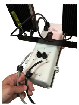
You may need to remove the RJ45 connector, and use a crimping tool to connect the Ethernet wires to an RJ45 connector inside the enclosure. Use an Ethernet cable of the width of  $5 \sim 6.5$ mm.
