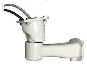
17. Mount the enclosure on to the installed bracket, and secure the connection by tightening the 4 socket screws. Due to the weight of the enclosure (5.5kg), it is best to have two men mounting the enclosure.
