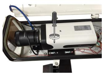
13. Attach the AC24V power wires and power inputs from the IR light units to the terminal connector. Connect the Brown and Orange (20AWG-thicker lines) wires from both IR units to the terminal. Since AC 24V is polarity free, Connect AC 24V from outer source, 24V inputs for IR (2 pairs), and 24V inputs for camera, all to the same terminal connector.
