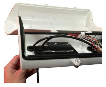
**8.** Prepare the AC24V power wires and a CAT5e Ethernet cable. Pass them through the waterproof connectors.
