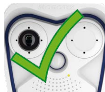
M15 with one blind module: Unrestricted operation (IP66)
