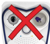
M15 with one transport plug: No operation allowed!
