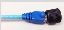
Unfit size of RJ45 Connector
