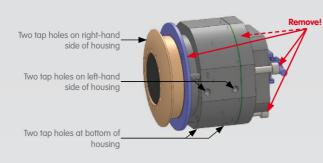
The housing can be installed by affixing suitable screws M4 (4 mm length of thread) in at least two of the six tap holes Remove pressure plate and cylinder head screws.
