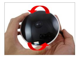
2. Insert the memory card into the card slot with the metal contacts facing the bottom side of the camera.
