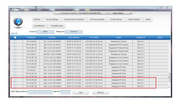
You can quickly see the camera model in the list. Click on the IP address to automatically launch the default browser of the PC with the IP address of the target camera filled in the address bar of the browser already.
