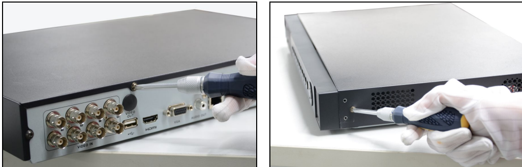
Figure 2. 1 Remove the Cover
