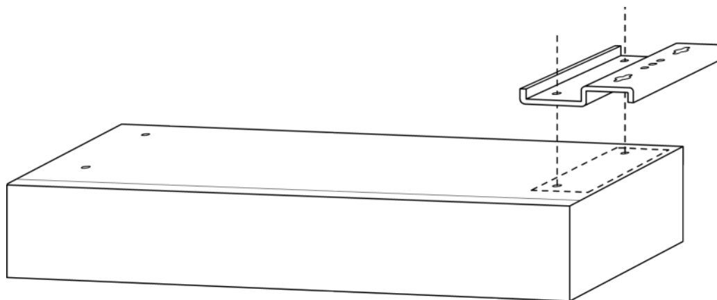
Figure 23: Position metal wall mount on bottom of E-Series
