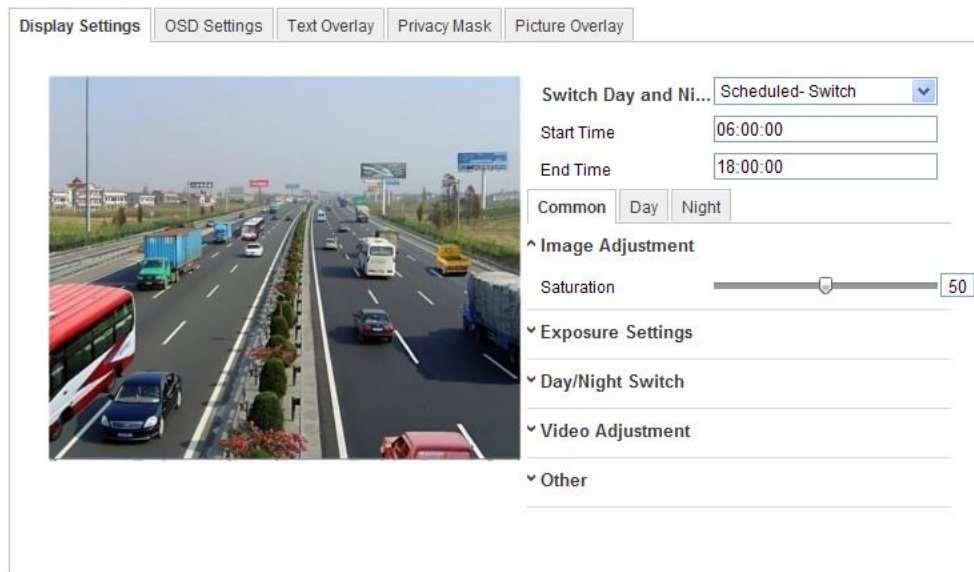
Figure 6-37 Day/Night Scheduled-Switch Configuration Interface
