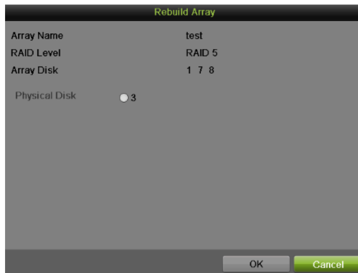
Figure 179 Rebuild Array Interface
