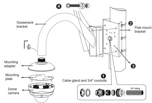
4. Secure the gooseneck bracket using the included hex bolts, washers, and nuts.
