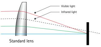
The problem can be rectified by using IR-corrected lens, which focuses both the visible and the infrared light in the same vertical plane.
