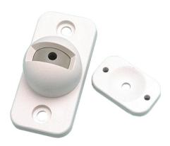
Surface-mount the plastic, low-profile mount to the wall. It is suitable for use with many detector types. The vertical swivel range is  $\pm 10^{\circ}$  to  $-20^{\circ}$ , while the horizontal swivel range is  $\pm 25^{\circ}$ .
