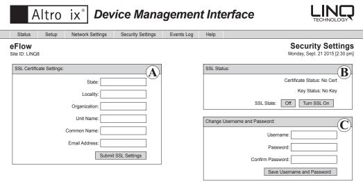
After all fields have been completed click [Submit SSL Settings] button, a dialog box will appear "Please allow up to 30 sec for server to reboot" click "OK". A self-signed SSL certificate will be generated with the information provided in the "SSL certificate settings" fields. The certificate will be valid for 500 days, and time stamped with the time settings present on the LINQ8PD(CB) module. The date and time must be synced with the host computer before generating an SSL certificate.
