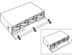
3 Align and push a bracket in the direction of the board
