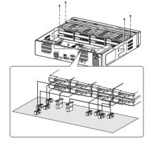
2 Remove the screws on the left/right side (4 screws) and remove the bracket.
