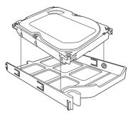
**X** How to exchange an installed HDD
