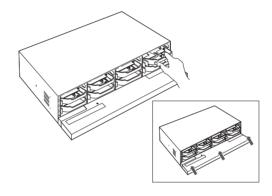
If you are adding a new or previously used HDD to this product in addition to the HDD(s) originally installed, format the new HDD manually in the set before use.
