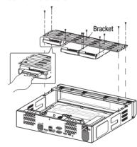
6 Check for any problems in the connection terminal and the wiring in the product, close the cover and fix it with screws.
