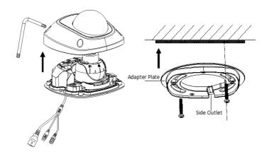
8. Use the supplied adjusting tool to adjust the pan [ $\pm 30^{\circ}$ ], tilt [0~80°], and rotation direction [0~360°].
