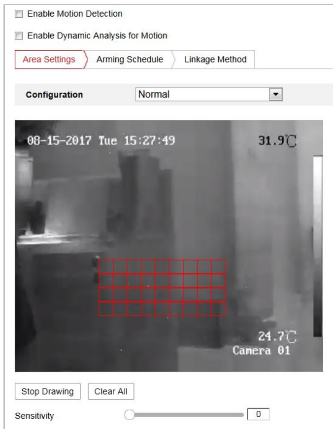
Figure 9-1 Enable Motion Detection
