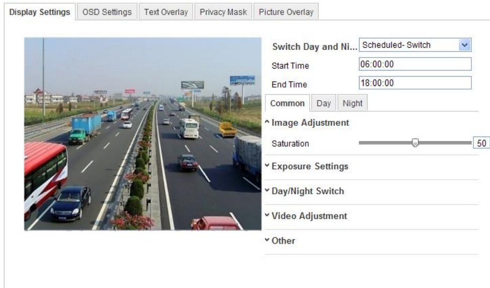
Figure 6-37 Day/Night Scheduled-Switch Configuration Interface
