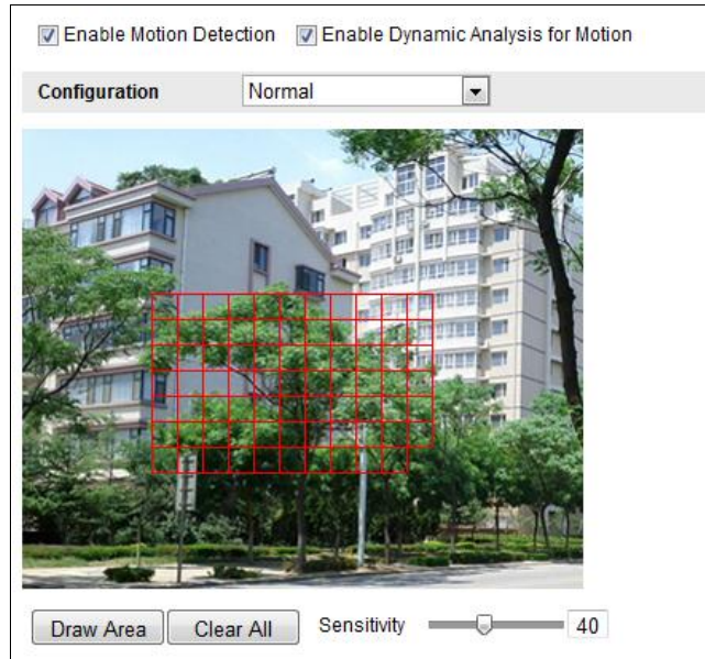
Figure 6-41 Motion Detection Settings-Normal
