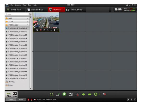
You can click the buttons on the toolbar to operate in the live view mode, e.g., capture picture, start/stop recording, two-way audio, PTZ control (with PTZ camera connected to the encoder), digital zoom, open/close audio, play back video files, etc.
