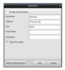
3. Edit a nickname for the device and input the IP address, port number (default: 8000), login user name (default: admin) and password (default: 12345) of the device.
