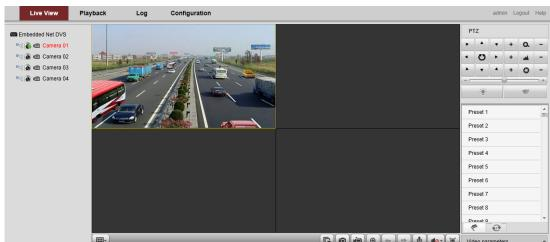
3. You can click the button on the toolbar to start the live view of all cameras on the device list.
