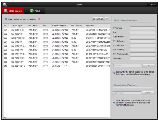
*Note:* Device can be searched and displayed in the list in 15 seconds after it goes online; it will be removed from the list in 45 seconds after it goes offline.
