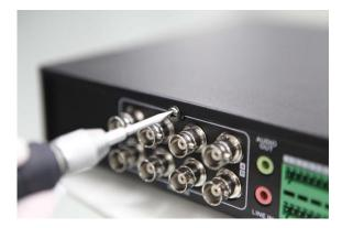
Place the HDD into the slot of the chassis and then secure it in position by fastening the screws at the bottom of the chassis.
