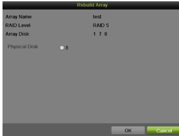
Figure 141 Rebuild Array Interface
