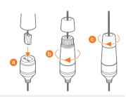
Note: To ensure moisture seal, make sure the o-ring is in place between (a) and (b). In extreme environments use of an outdoor rated sealer is recommended.
