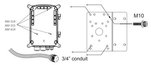
The mounting hole definition is illustrated below. The same mounting hole pattern apply to all pole-mount and corner-mount brackets.
