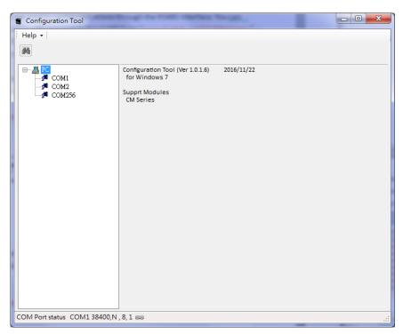
1. First select the correct COM port that is connected to CaMate.
