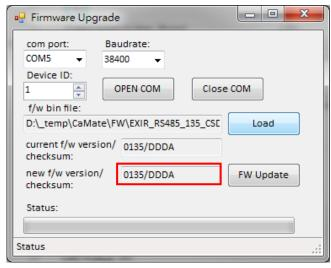
3. Click FW Update and confirm the upload, firmware upgrade will then start. Please do not turn off the power to CaMate untill the upgrade is completed.
