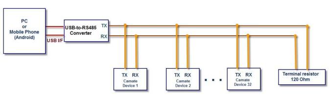
NOTES: If termination is required, a resistor value of  $120\Omega$  or greater should be used, and no more than 2 termination resistors should be used, one at each end of the RS485 transmission line.
