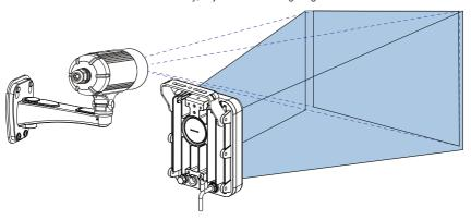
Turn the illuminator toward the FOV of the partner camera, shift the tilt angle, and then tighten the screw to secure the illuminator.
