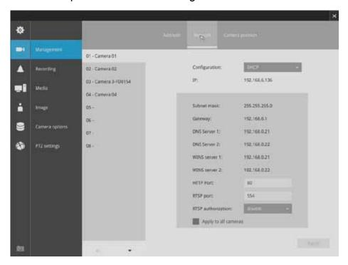
You can select DHCP as the method for cameras to acquire IP addresses, or you can manually configure static IPs for a single or all cameras. Using static IPs is recommended. Although the NVR can remember the MAC addresses of cameras, if IPs are changed under the DHCP configuration, your NVR may still fail to connect the cameras. Please consult your network administrator for details about network settings.
