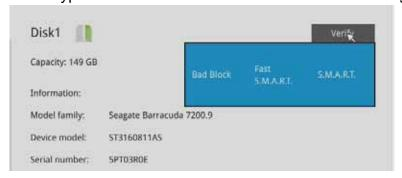
**Bad block check**: Performs read/write test to drive sectors to locate bad blocks. This action may take several hours to complete.
