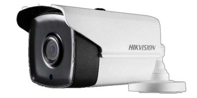
The Hikvision DS-2CE16D7T-IT5 is a 2 megapixel bullet camera that offers high definition (HD) analog video at 1080p resolution over existing coaxial cables.
