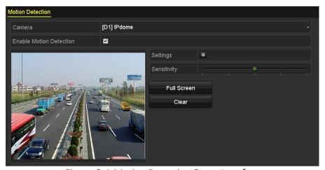
Figure 8-1 Motion Detection Setup Interface
