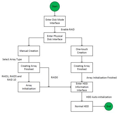
Figure 13-1 RAID Working Flow
