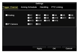
Figure 9-15 Set Trigger Cameras of POS
