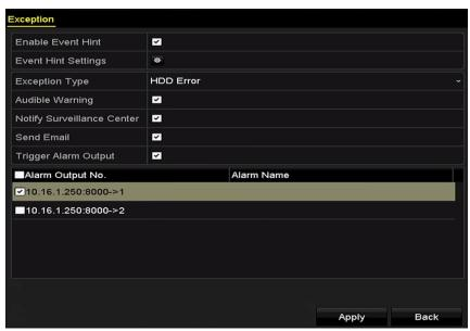
Figure 14-30 Configure HDD Error Alarm
