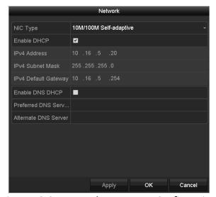
Figure 12-24 Network Parameters Configuration
