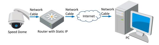
Figure 2-10 Accessing the Mini PTZ camera through Router with Static IP
