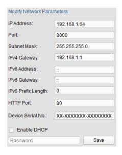
Figure 2-5 Modify the IP Address
