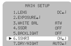
2. Select a desired mode using the Function Setup switch.
