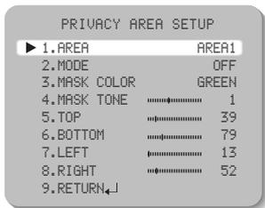
1) When the SPECIAL menu screen is displayed, press the Function Setup switch so that the arrow indicates 'PRIVACY'.
