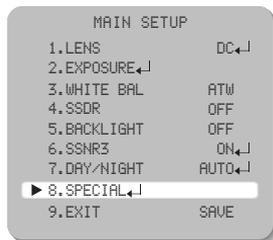
2. Select a desired mode using the Function Setup switch.
