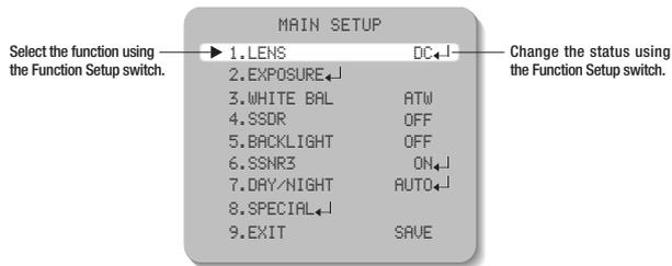
2. Select a desired function using the Function Setup switch.
