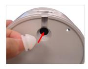
2. Run the cable (without adapter) through the wall mount and secure the wall mount to the wall using the (4) wall mount screws.
