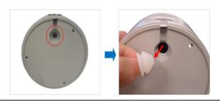
d) Slightly cut off the tip of the rubber, just enough for the rubber to expand and let the Ethernet cable to pass through.
