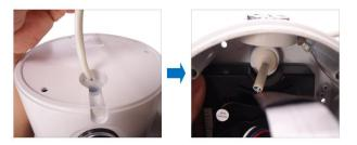
7. Once the cable length is determined (able to reach camera Ethernet port), seal the bottom cable hole with silicone to protect it from water leak.
