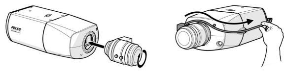
c. Connect the auto iris cable to the 4-pin connector located on the back of the camera.
