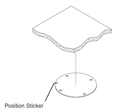
Apply the position sticker to the desired camera mounting position.
