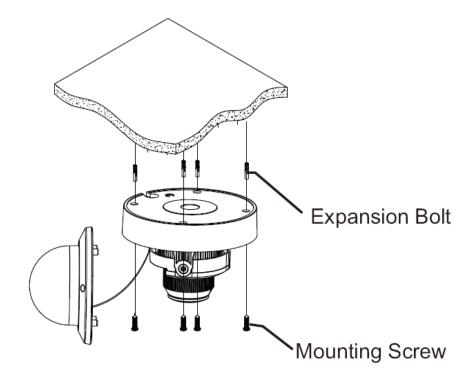
Use the position indicated on the position sticker to drill the holes needed to mount the camera base. Insert the expansion bolt into the holes. Match the base's mount openings to the expansion bolts position, and then place the mounting screws through the base's mount opening into the expansion bolt. Tighten the mounting screws to ensure the camera base mounted securely.
