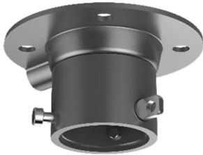
The mount must be installed on a flat wall. Waterproof rubber is necessary for outdoor application. The wall must be capable of supporting at least three times as much as the total weight of the camera and the mount. The mount's maximum load capacity is 44 lbs (20 kg).
