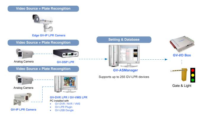
Note: Edge GV-IP LPR Camera includes GV-LPR2811-DL / GV-LPR2800-DL / GV-LPR1200.
