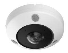
CMIP7112F-SE is a fisheye network camera capable of providing a 360-degree panoramic image of its scene. The progressive scan CMOS sensor provides high-resolution images of up to  $3504 \times 3504$ . Up to 20 live view display modes, designed for 3 mount types, meet various user preferences. Three independently controlled IR lights offer a range of 15 m and provide good vision in low or even zero-light environments.
