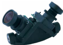
2 lens units on lens bridge 180°
