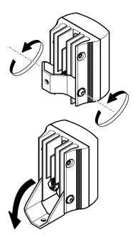
3. If required, loosen the screws and change to a diverging lens with the desired angle of illumination. The angle of illumination should be adjusted according to the camera field of view to light the whole scene adequately. See Technical Specifications.
