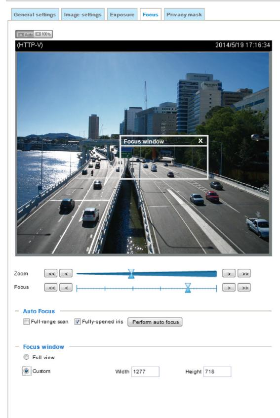
Perform the Auto Focus function for best image. However, if you have cascaded cameras, do this one by one. Do not perform this function simultaneously on multiple cameras because the motorized lens also consume considerable power, and may cause the last camera on the line to hang.
