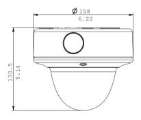
Dimensions in mm (in.) for surface mounting
