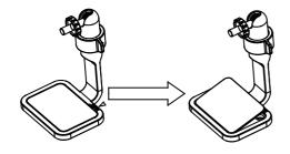
2. Drill the screw holes according to the drill template.
